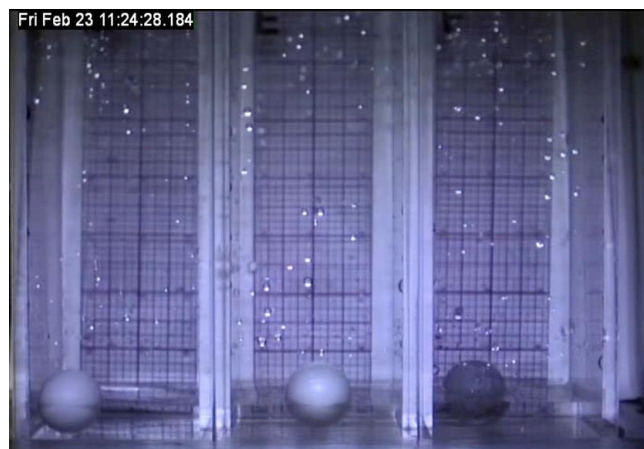
Fig. 9. Experiment 2 – Test objects position in the test cell AFTER the drop into microgravity, the droplets on the container are from previous tests, (from left to right PTFE; Paraffin coated PTFE; and butyl rubber coated PTFE objects).
